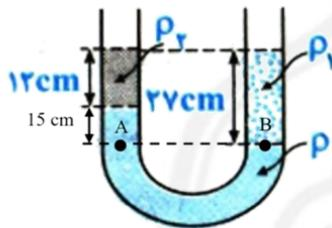
$$\begin{aligned} p_A = p_B &\Rightarrow p_0 + \rho_1 gh_1 + \rho_2 gh_2 = p_0 + \rho_1 gh_1 \\ &\Rightarrow \rho_2 h_2 = \rho_1 h_1 \\ &\Rightarrow \rho_1 = \frac{\rho_2 h_2}{h_1} = \frac{(1.24)(15) + (1)(12)}{27} = 1.13 \frac{\text{g}}{\text{cm}^3} \end{aligned}$$
